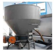
BMS alpha Z3 Styrofoam may equally be equipped for conveying cement screed.
