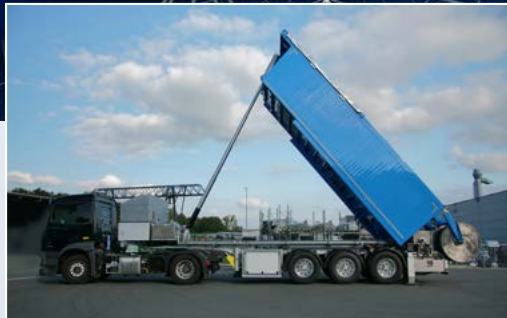
Tilting system for fluid screed. TITAN F. Compact machine technology, powerful performance.
