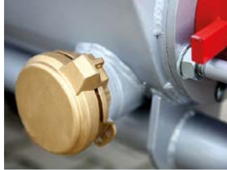
Large opening for cleaning
