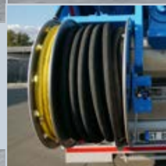
Hose reel (hydraulic driven) positioned in the rear.
