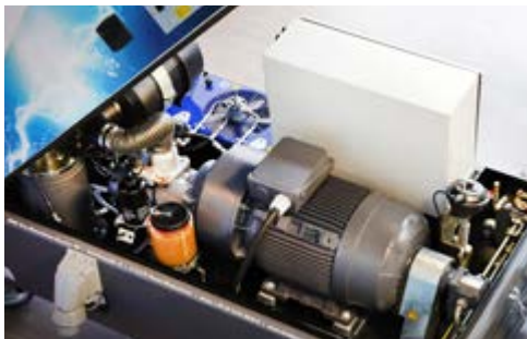
The 30 kW variable frequency electric motor
