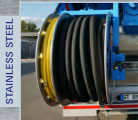
Hose reel (hydraulic driven) positioned in the rear.
