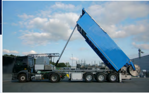
Tilting system for fluid screed. TITAN F. Compact machine technology, powerful performance.
