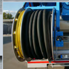
Hose reel (hydraulic) positioned in the rear.
