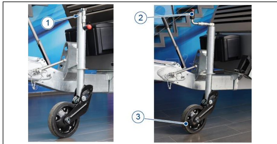
Figure 29: Turn the support wheel upwards
