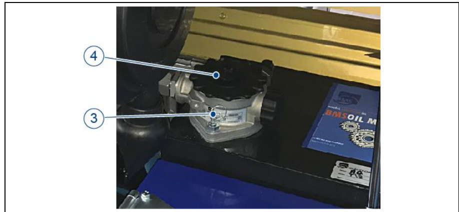
Figure 44: Check hydraulic oil level
