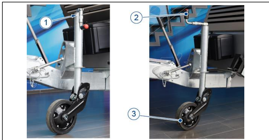
Figure 24: Turn the support wheel downwards
