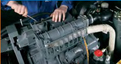
The 4-Cylinder-Diesel engine with max. 48.5 kW.
